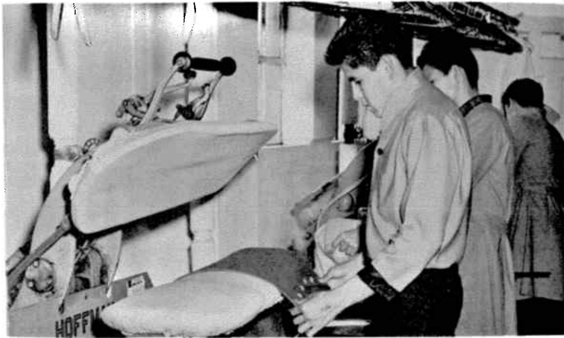
In preparation for the finisher, Ceed Cheschilly is shown blocking a dress on the utility press.
