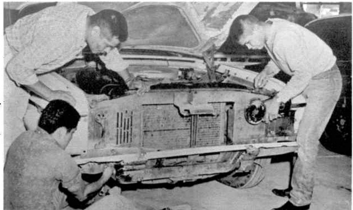
Mr. James Larney observes the work of Luther Tahy, left; and Riley Saganitso, right; as they line up the front panels on a '63 Ford convertible.
