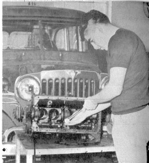
Alvin McClure checks a main bearing on an engine.
